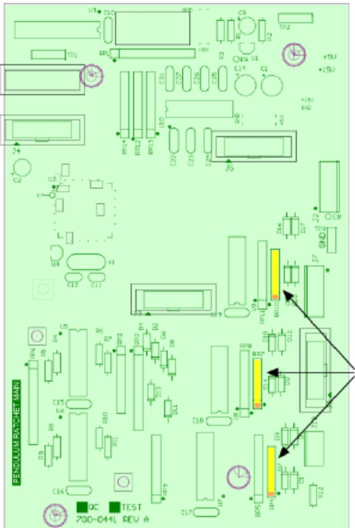
Three resistor packs determine output pulse voltage. This is a drawing of the component side of the main board.
