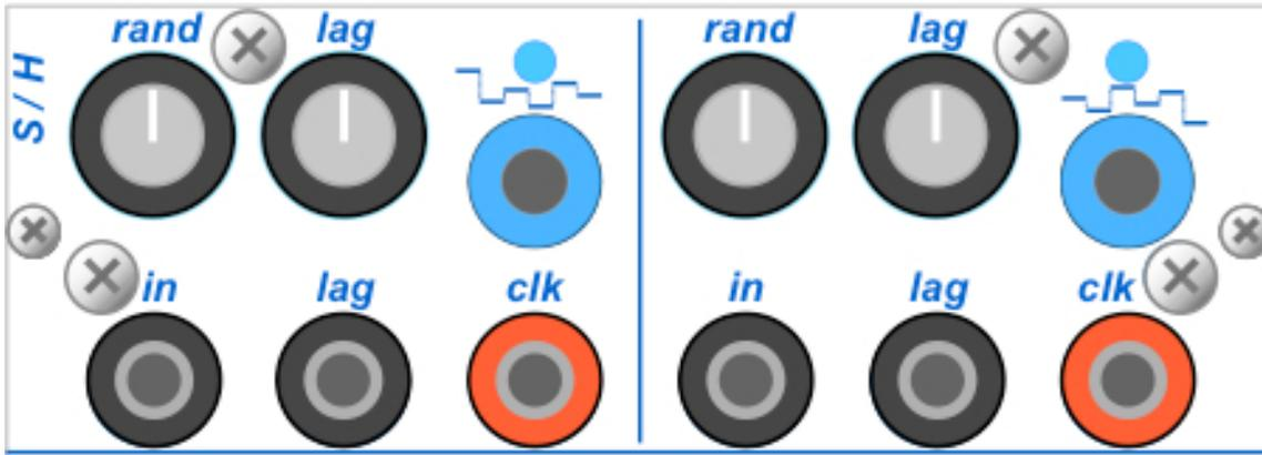
The Sample/Hold has two inputs: a CV from the In jack, and a random voltage amount set on the Rand knob. The output of the Sample/Hold goes into a Lag section, which slows down the rate of change. This Lag can be voltage controlled.
